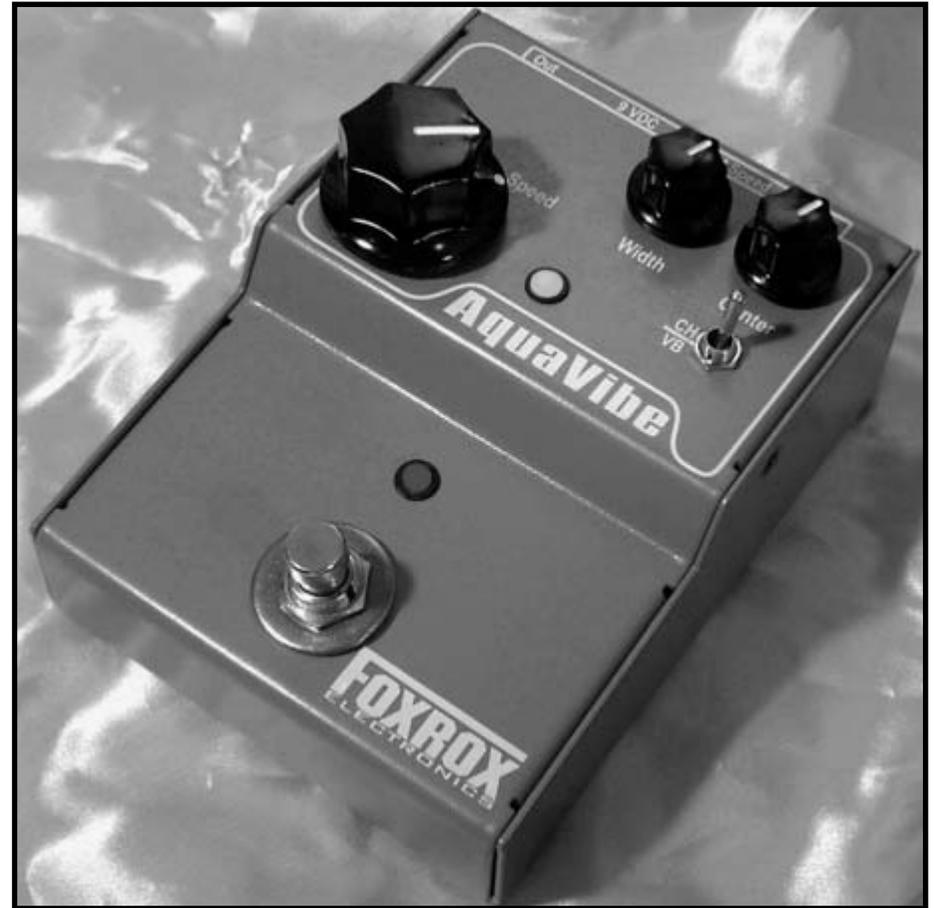
Temperature - Always allow Aquavibe to achieve room-temperature for best results. The photocells used for phase shifting and speed control are affected by temperature. If you bring Aquavibe in from the freezing cold it might not sound right until it's allowed to warm up.
